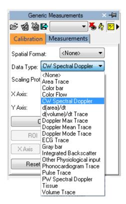
Next, establish (using the X axis and the Y axis) the calibration values to be assigned to the image. For instance, in case of a Doppler image, assign a time value on the X axis and a speed value on the Y axis. For 2D images, which have the same unit of measurement for both axis, it is also possible to calibrate both axis at once with a single diagonal segment using the *Both* button.
